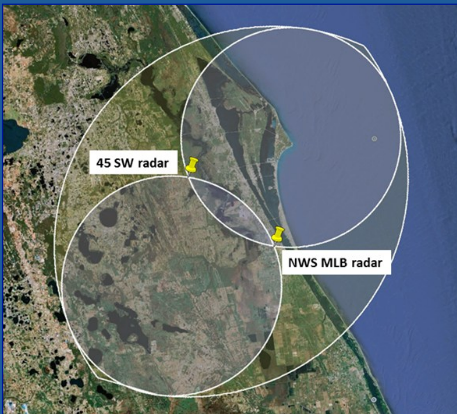
Figure 10. The total coverage area for the 45 SW and NWS MLB radars. The yellow pins show the locations of the radars.
