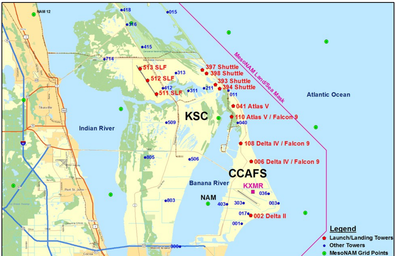
Figure 12. Map of KSC/CCAFS showing the wind tower locations as red pentagons labeled with tower number and the supported launch activity, MesoNAM model grid points as green circles, and the CCAFS weather station as a magenta square labeled KXMR (Bauman 2010, Figure 1).
