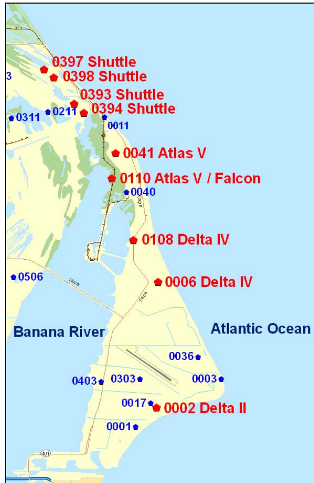
Figure 7. Map of KSC/CCAFS showing the locations of the mesonet wind towers. The onshore and offshore stratifications were determined by the coastline alignment relative to the Atlantic Ocean for each tower.
