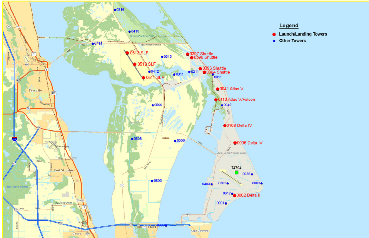
Figure 5. Map of KSC/CCAFS showing the locations of the wind towers used to verify MesoNAM forecasts. The verification tower locations are indicated by red pentagons and labeled with tower number and supported launch activity.
