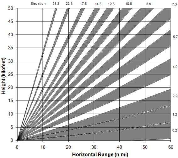
Figure 7. Range-height cross section of beam coverage for the 45 WS scan strategy using the elevation angles listed in Table 2.
