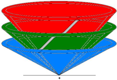
Figure 3. A 3-D schematic representing the radar coverage by provided by three  $360^{\circ}$  scans with antenna elevation changes shown as grey ramps.
