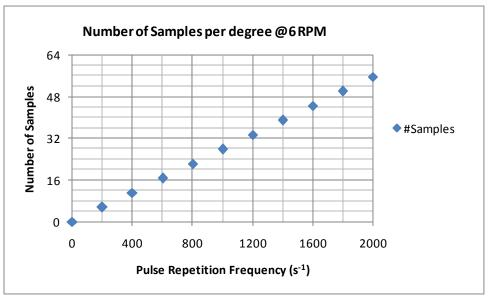
Figure 11. Number of samples per one-degree azimuth interval versus pulse repletion frequency, for an antenna rotation rate of 6 revolutions per minute.
