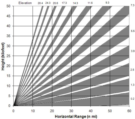
Figure 8. Range-height cross section of beam coverage for the AMU scan strategy, based on the current WSR-74C strategy, with one additional elevation angle.
