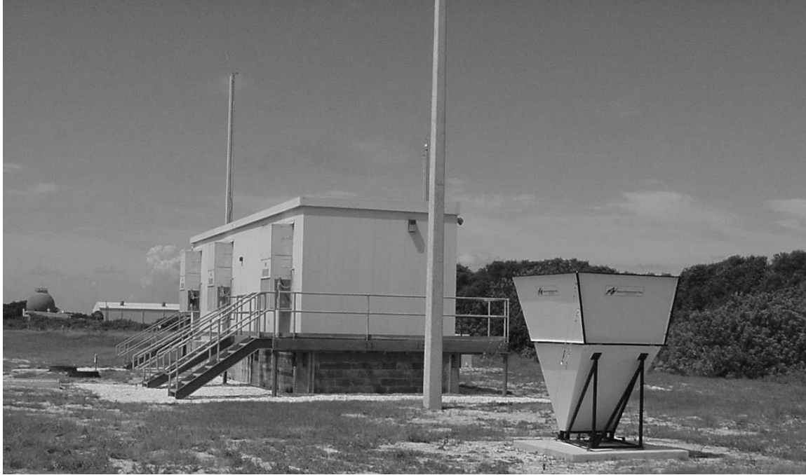
Figure 2. Photograph of DmSS site and nearby building. The DmSS and building are separated by about 40 ft. A 2-lane road runs parallel to the front of the building approximately 60 ft to the left. The DmSS site includes a sonic anemometer on a 33 ft (10 m) pole that is behind the building and partially obscured from view by the pole in the foreground. Sonic anemometer data are integrated into the DmSS data stream.
