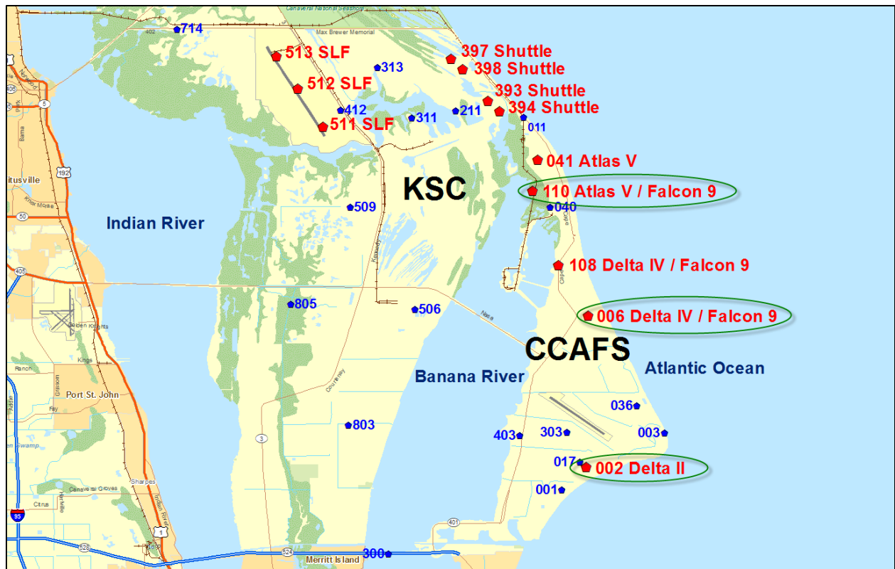
Figure 9. Map of KSC/CCAFS showing the locations of the wind towers used to verify MesoNAM forecasts (red pentagons labeled with tower number and the supported launch activity) and the dual-sensor towers (green ellipses). The onshore and offshore stratifications were determined by the coastline alignment relative to the Atlantic Ocean for each tower.
