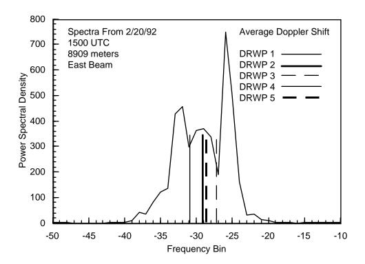
Figure 4.46. East beam spectral estimates from the 8909 meter level at 1500 UTC on 20 February 1992. Identical line types are used for identical or nearly identical average Doppler shifts.
