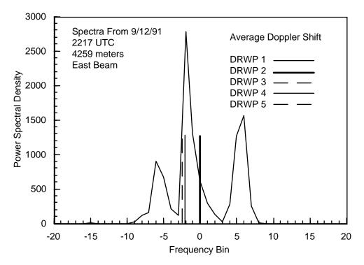
Figure 4.34. East beam spectral estimates from the 4259 meter level at 2217 UTC on 12 September 1991. Identical line types are used for identical or nearly identical average Doppler shifts.
