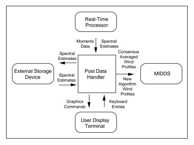
Figure 3.12. External interfaces of the Post Data Handler. The control and data flows between the User Interface Function and other components of the DRWP are illustrated in Figure 3.13. Data input into the User Interface Function include:
