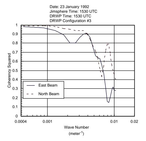
Figure 4.15. Coherency analysis of jimsphere and MSFC wind algorithm DRWP profiles for 23 January 1992. Profile times are: Jimsphere 1530 UTC and MSFC wind algorithm 1530 UTC.
