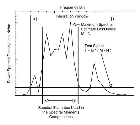
Figure 3.3. Example of the relationship among the test signal, T, the maximum spectral estimate within the first guess window less the noise, M - N, the integration window width, and the spectral estimates used in the spectral moments computations.
