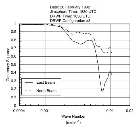
Figure 4.29. Coherency analysis of jimsphere and MSFC wind algorithm DRWP profiles for 20 February 1992. Profile times are: Jimsphere 1830 UTC and MSFC wind algorithm 1830 UTC.
