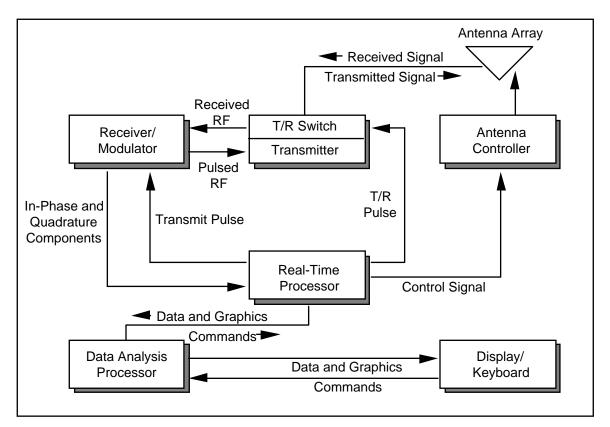
Figure 1.2. Simplified block diagram for NASA's 50 MHz DRWP.
