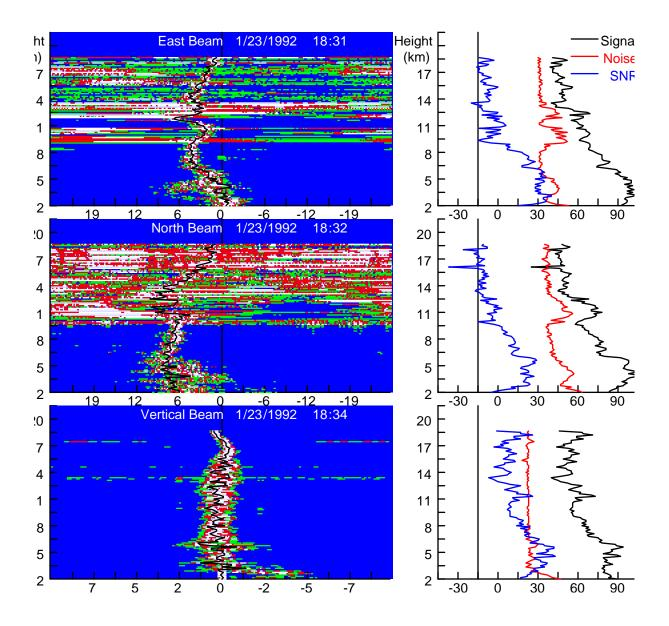
Figure 4.20. Example of spectral data contaminated by lightning. Spectral estimates for the east, north, and vertical beams are color coded and overlaid with the radial velocity estimates (black trace). Relatively larger spectral estimates are coded white while relatively smaller spectral estimates are coded blue. The units on the horizontal axis of the spectral estimate displays are m/s. The units of the corresponding signal, noise, and SNR profiles are decibels.
