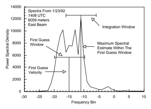
Figure 3.2. Example of how the first guess velocity, the first guess window width, and the integration window width are used to compute the spectral moments.
