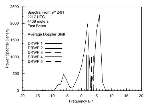
Figure 4.35. East beam spectral estimates from the 4409 meter level at 2217 UTC on 12 September 1991. Identical line types are used for identical or nearly identical average Doppler shifts.
