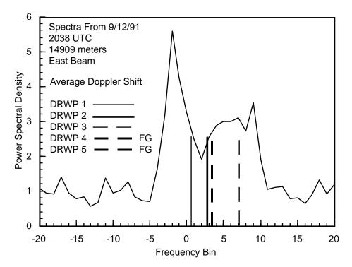
Figure 4.33. East beam spectral estimates from the 14909 meter level at 2038 UTC on 12 September 1991. FG indicates the first guess velocity was
