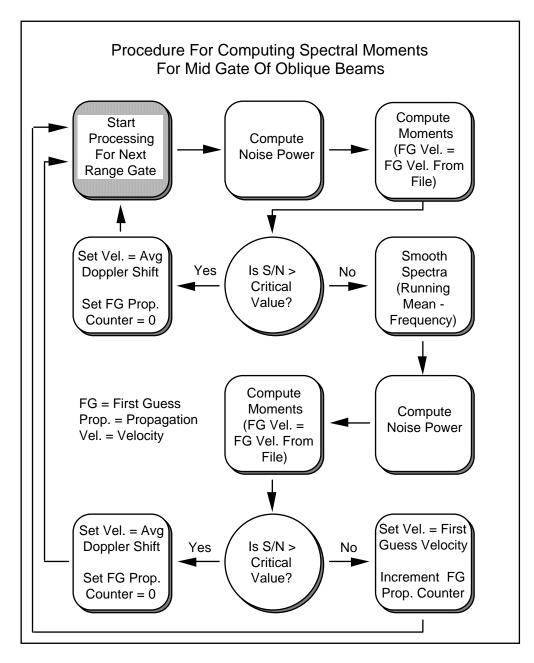
Figure 3.5. Procedure for computing the spectral moments for the mid gate of the oblique beams.
