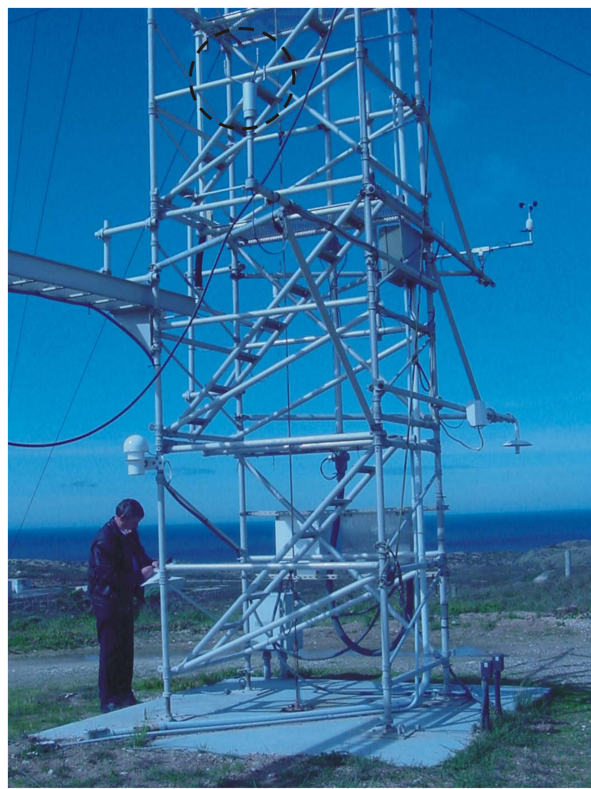
Legacy and RSA wind sensors at the 12 ft level on Tower 102 at VAFB. Legacy cups can be seen in the middle-right. The Legacy wind vane is obscured by the electronics box. The RSA1 ultrasonic sensor can be seen in upper-center, inside the dashed black circle.
